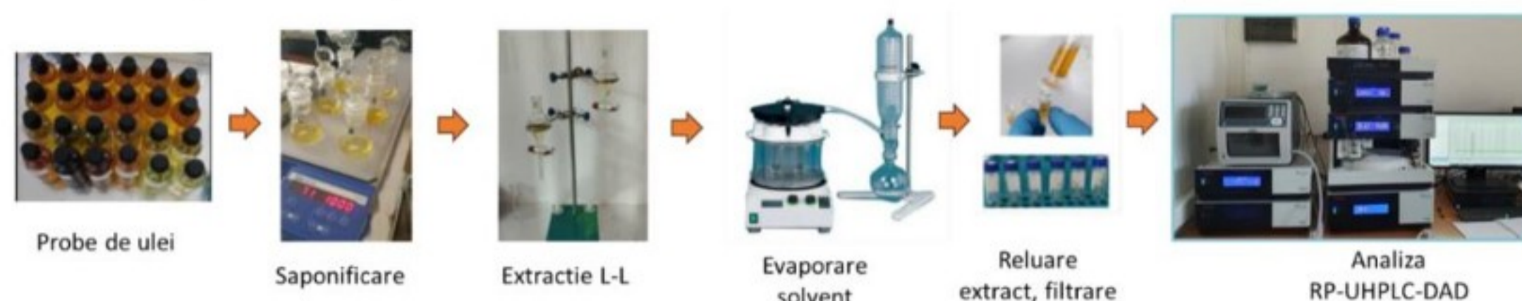
Figure 1. Schematic representation of the extraction of sterols and triterpene diols from vegetable oils before analysis by RP-UHPLC-DAD
